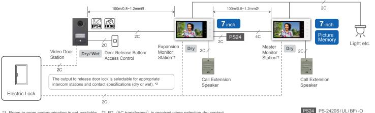
\*1. Room to room communication is not available. \*2. PT (AC transformer) is required when selecting dry contact.
